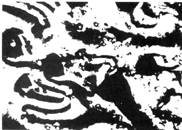
Figure 2. Microphotograph of a sample of 6j between crossed polarizers at 262 °C at a magnification of 2773.
